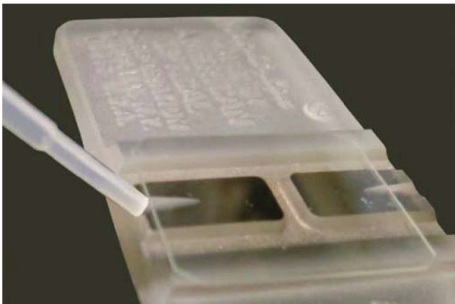
Figure C-6. A pipet is used to load the hemocytometer. Care must be taken to maintain a steady flow of fluid until the chamber is fully charged but not overflowing into the moat.
