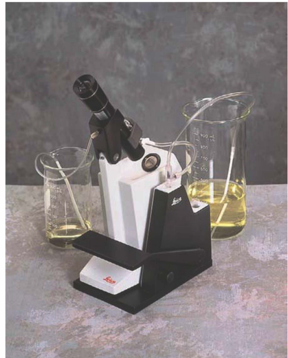
Figure 7-6. Total solids refractometer using flow-through setup.
