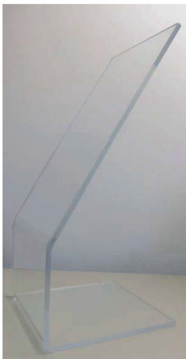
Figure 4-5. A table-top safety shield is one engineering device that can be used to protect personnel when handling specimens or chemicals.
